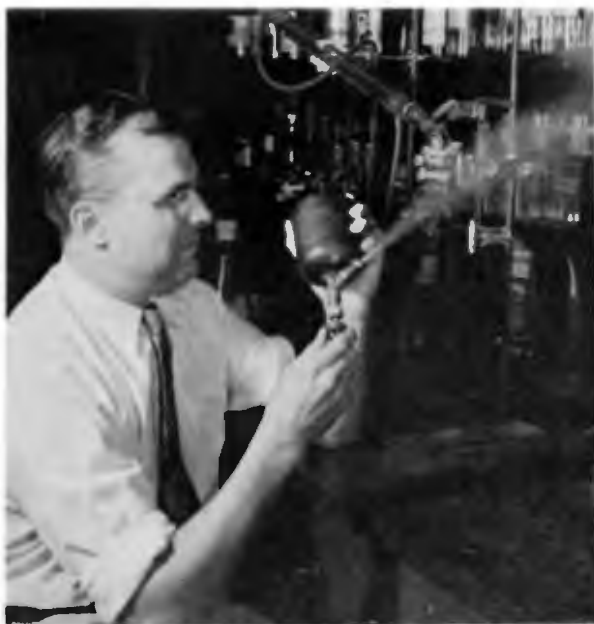
The author in the laboratory at Beltsville, Md. At left is the first 2D aerosol bomb ever made. At right is the filling equipment used.
